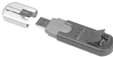
Picture 13. A compact USB network adapter connects directly into the USB port on a PC (Photo courtesy of Cisco System, Inc.)
