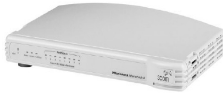
Picture 3. An eight port Ethernet hub
