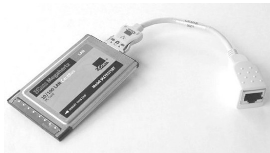
Picture 9. An Ethernet PC Card (PCMCIA) type network adapter and a dongle connector
