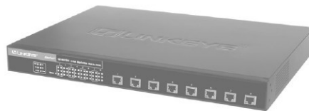
Picture 4. An eight port Ethernet switch
