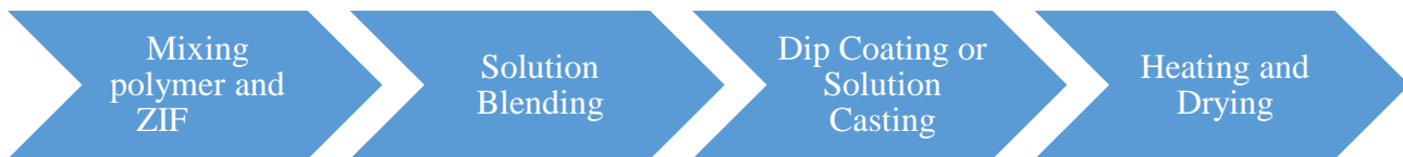
FIGURE 13. The MMMs' synthesis process (Chen et al. 2014, 9)
