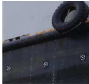
Fig. 2: The mobile optical TRITOP SM system in use at a dry-dock. System and accessory can be easily transported by a single person. The system can be operated during measurement and evaluation without external power supply
