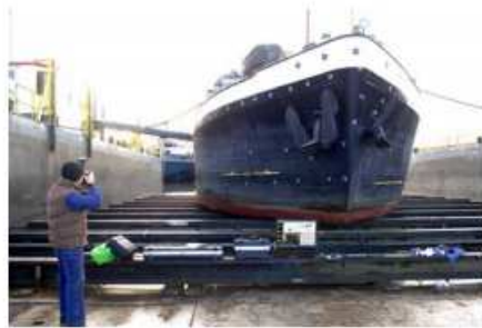
Fig. 2: The mobile optical TRITOP SM system in use at a dry-dock. System and accessory can be easily transported by a single person. The system can be operated during measurement and evaluation without external power supply
