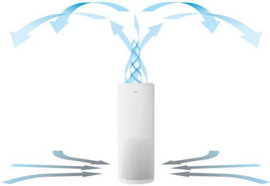
FIGURE 9. Diagram of how LA500 delivery clean air (adapted from LIFA air official website)
