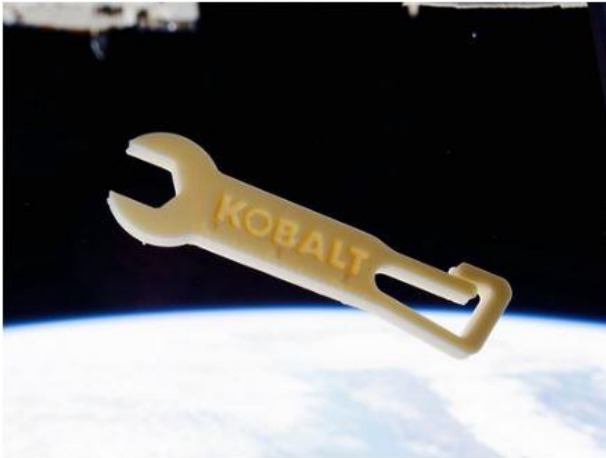
Figure 15. First 3D printed wrench in space (Lowe'sInovationLabs, 2016)
