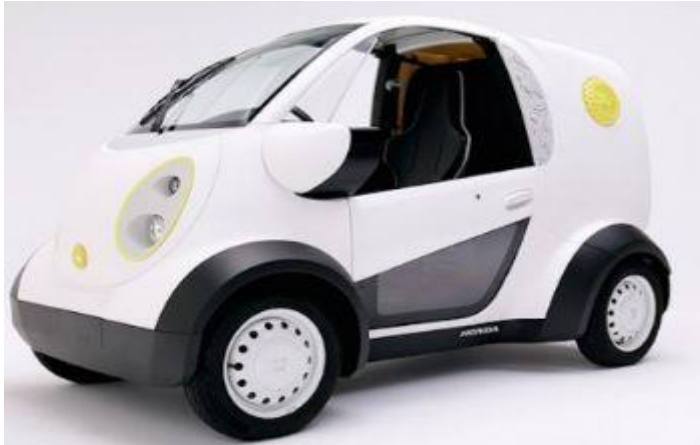
Figure 14. 3D printed Honda electric car (Patni, 2016)
