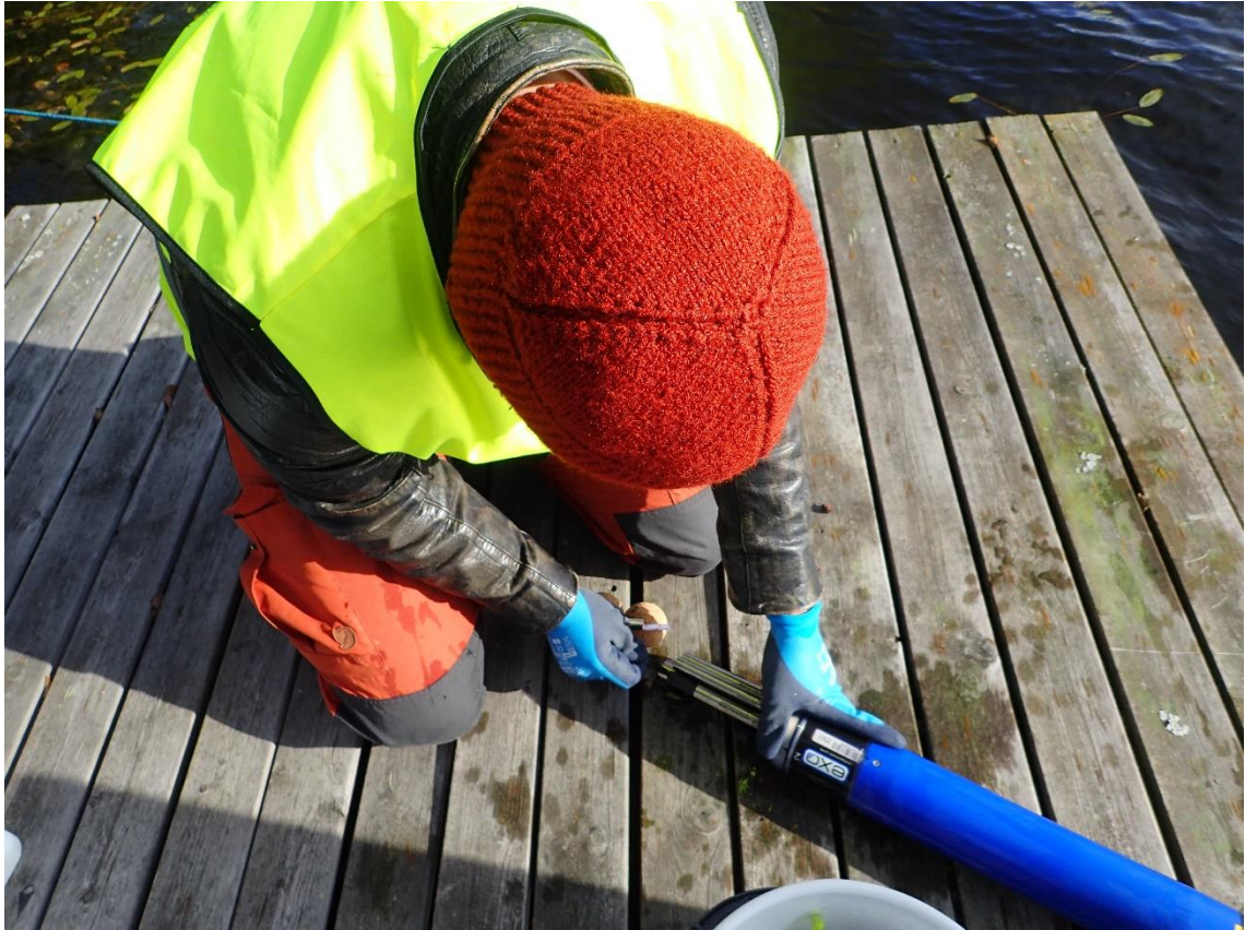
Figure 7. Maintenance work on the EXO2 sonde (image credit: LUVY)
