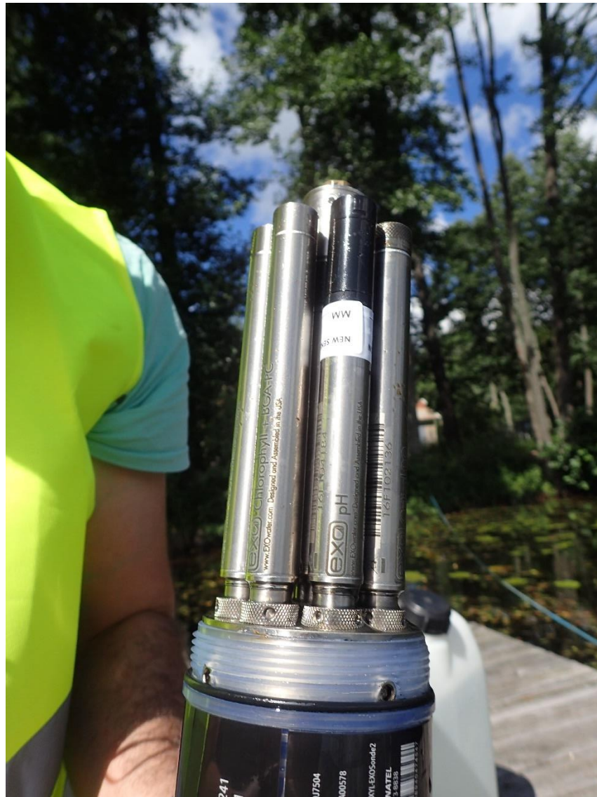
Figure 8. EXO2: a digital multiparameter sonde (image credit: LUVY)
