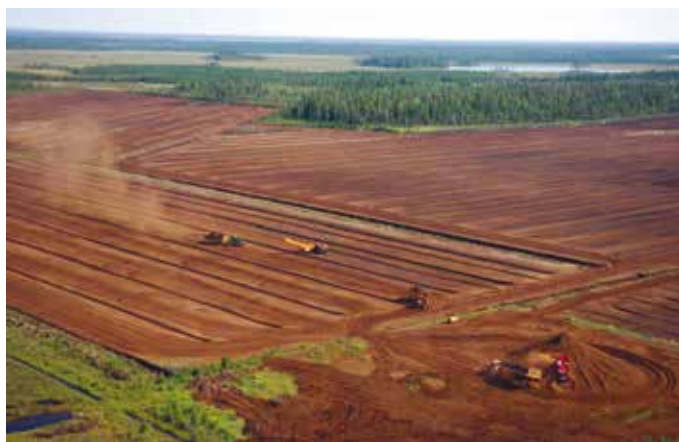
FIGURE 14. Haku -method's machinery. Milled peat loading, transport and adding to a stock pile. (Turveruukki Oy).
