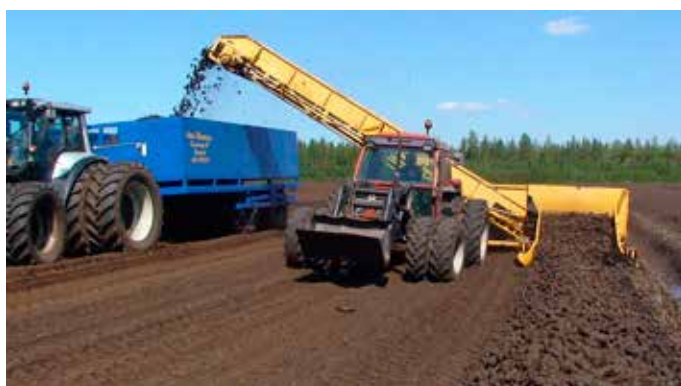
FIGURE 33. Sod peat loading with a conveyor belt loader (Suokone Oy).
