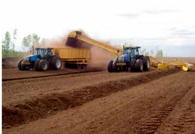
FIGURE 21. Loading peat in Haku -method (Suokone Oy).
