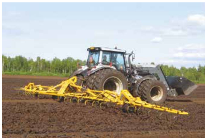
FIGURE 32. Harrowing disconnects the lowest sods from the field and speeds up drying (Suokone Oy).
