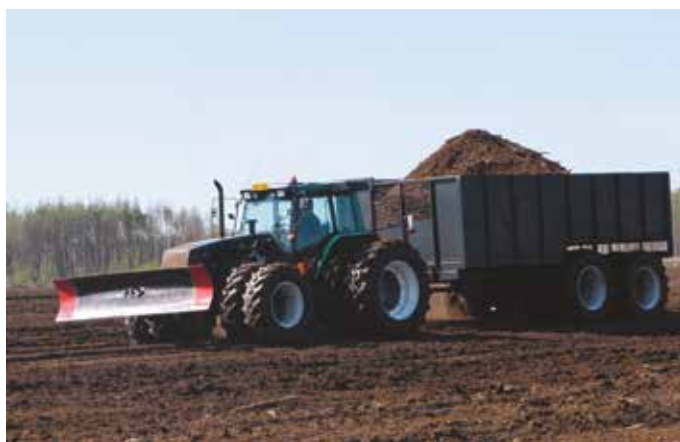
FIGURE 22. Transporting peat to the stock pile in the Haku -method (Tero Vesisenaho).
