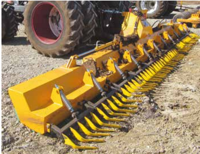
FIGURE 17. Knife-miller is suitable for fields where the peat layer getting shallow, also for highly decomposed peat. (Tero Vesisenaho).
