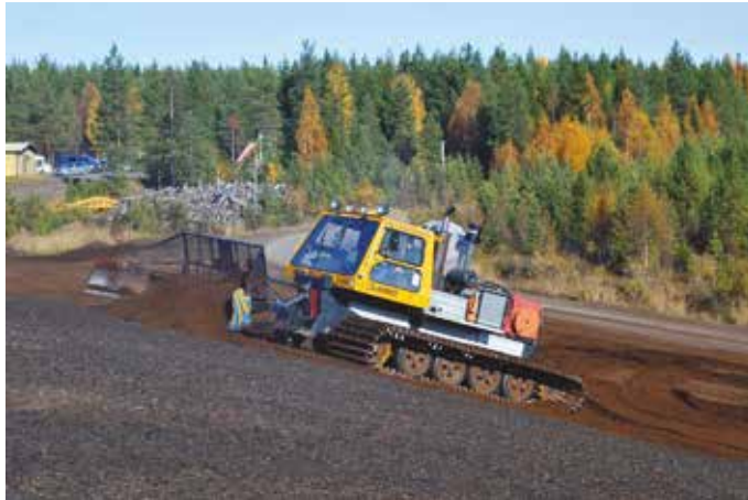
FIGURE 34. Stockpile making by pushing up can be also carried out with a snowcat (Vapo Oy).
