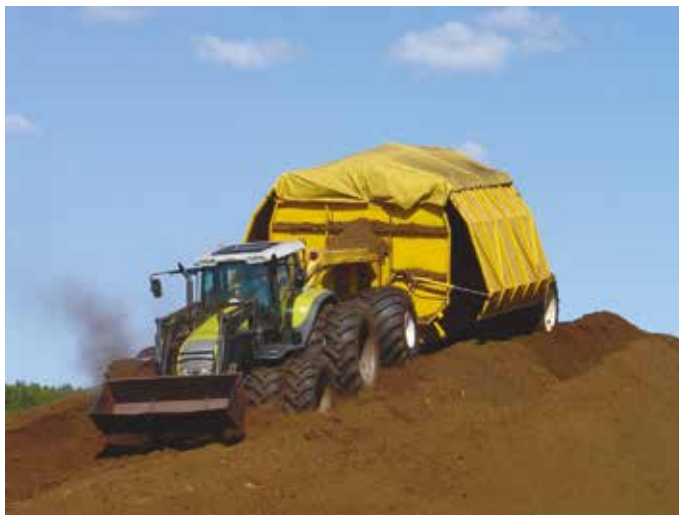
FIGURE 35. Drive-over stockpile is made by driving the peat transport vehicle over the stockpile and then emptying the load on the top of the stockpile (Turveteollisuusliitto Ry).
