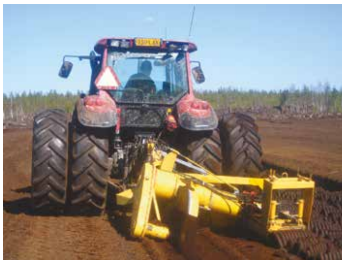
FIGURE 28. Sod peat shaping with wave-like sod peat nozzles (Mari Juntunen).
