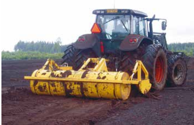
FIGURE 8. Maintenance miller (Suokone Oy).
