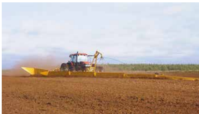
FIGURE 20. Milled peat ridger, also known as ruler-ridger (Turveruukki Oy).
