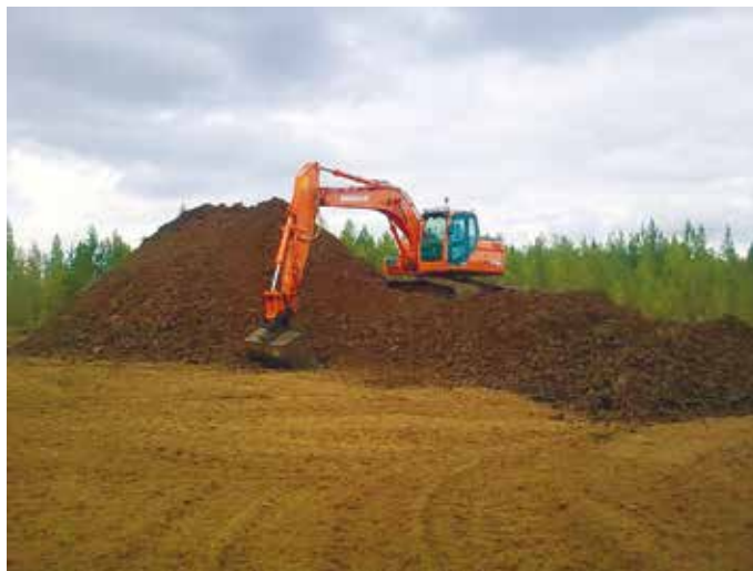
FIGURE 36. Stockpiling unscreened sod peat with an excavator (Mari Juntunen).
