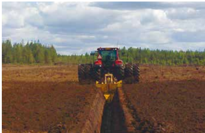
FIGURE 7. Ditch miller (Mari Juntunen).
