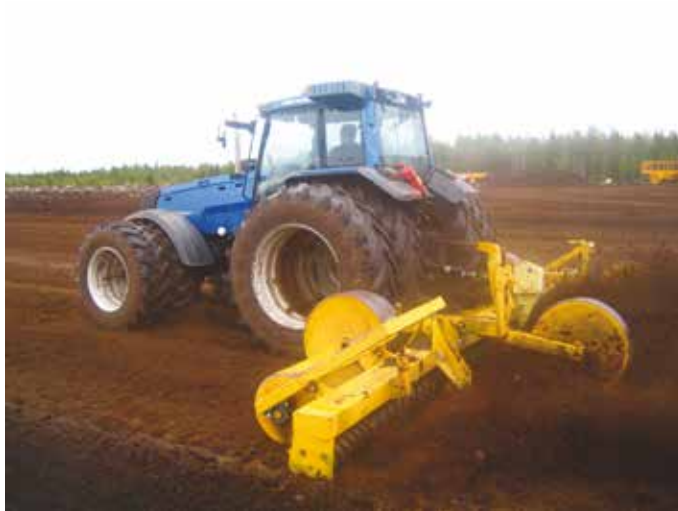
Figure 16. Powered miller breaks up the peat by milling (Mari Juntunen).
