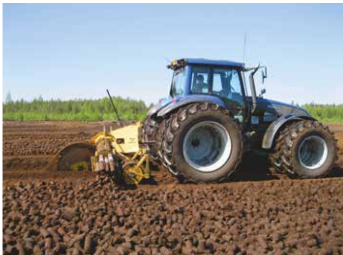
Figure 27. Sod peat shaping with cylinder extrusion nozzles (Laura Vertainen).
