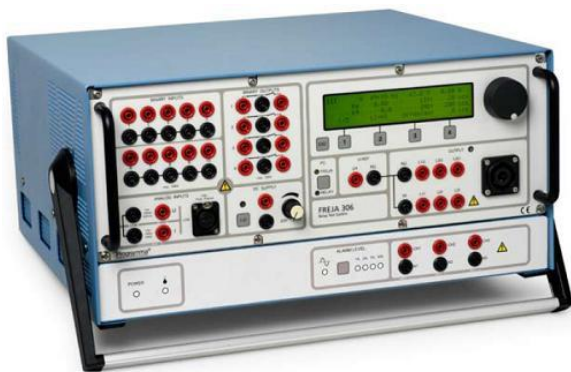
Figure 14: Freja 306, relay testing tool
