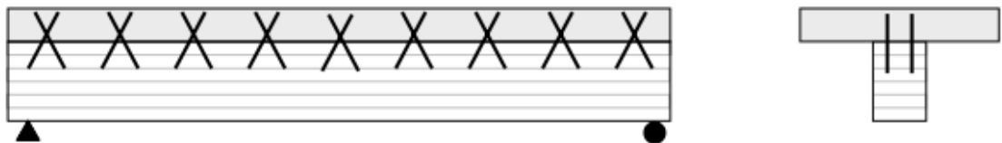
Figure 4. The principle of joining a timber beam and a concrete deck by using glued-in steel bars. (11)
