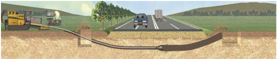
Figure 3.8 Pilot well expansion.
