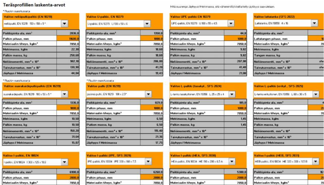
Figure 27. The steel profile selection tool uses a database in another sheet.
