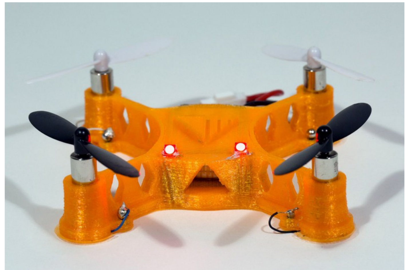
Image 36: 3D Printed Drone Printed on Voxel8's 3D Electronics Printer - Mashable - 2016
