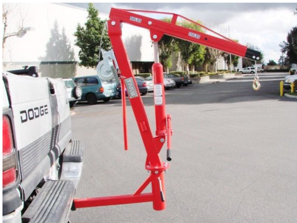
Figure 2 A hydraulic hoist by used in a trailer (TMS, 2016)
