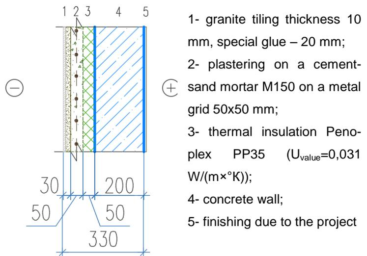
Figure 22. External wall section
