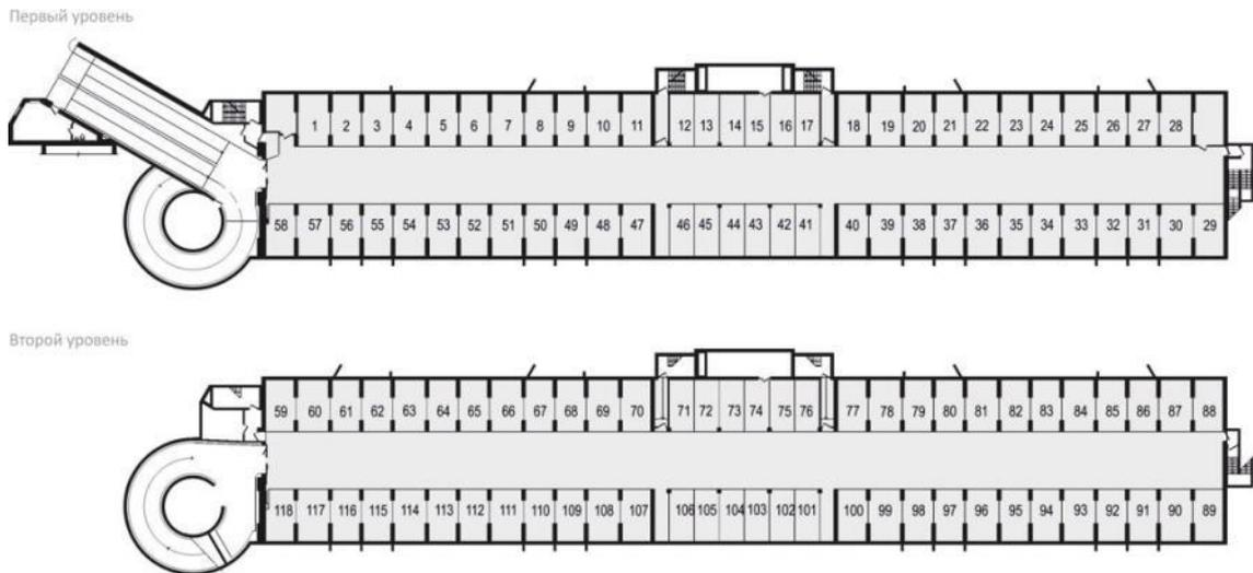
Figure 8. Multistorey parking of corridor type
