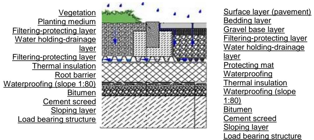
Figure 12. Inverted roof section. Lawn and driveways.
