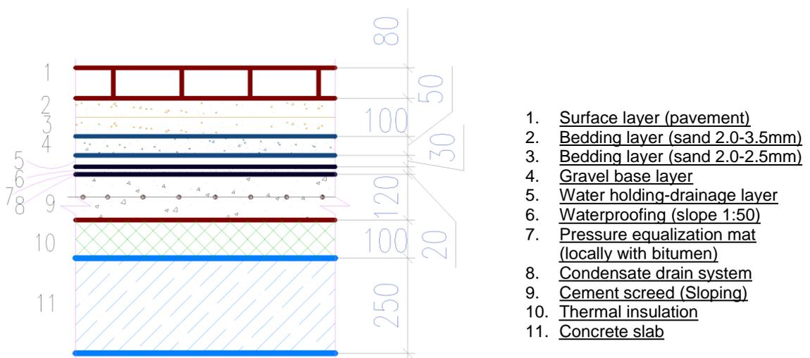
Figure 29. Walkways roof section
