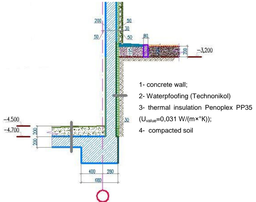
Figure 23. External wall section (parapet wall)
