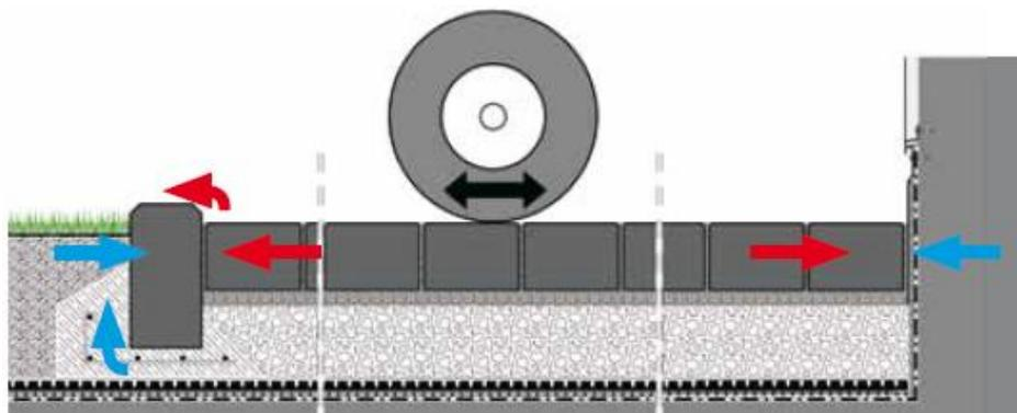
Figure 15. Steering, breaking and accelerating ([www.zinco-greenroof.com](http://www.zinco-greenroof.com))
