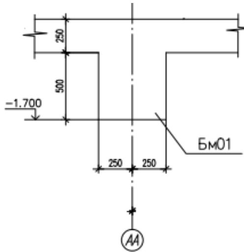
Figure 21. The section of parking roof slab
