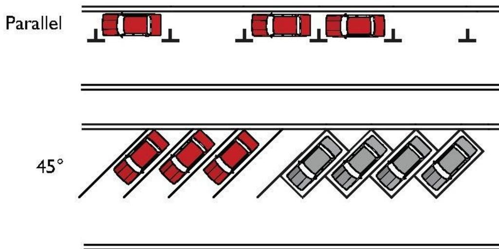
Figure 3. Single level parking of corridor type
