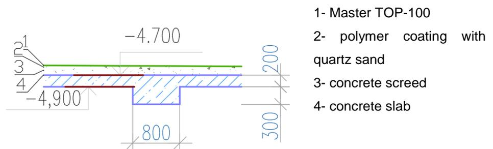
Figure 20. Section of the foundation slab
