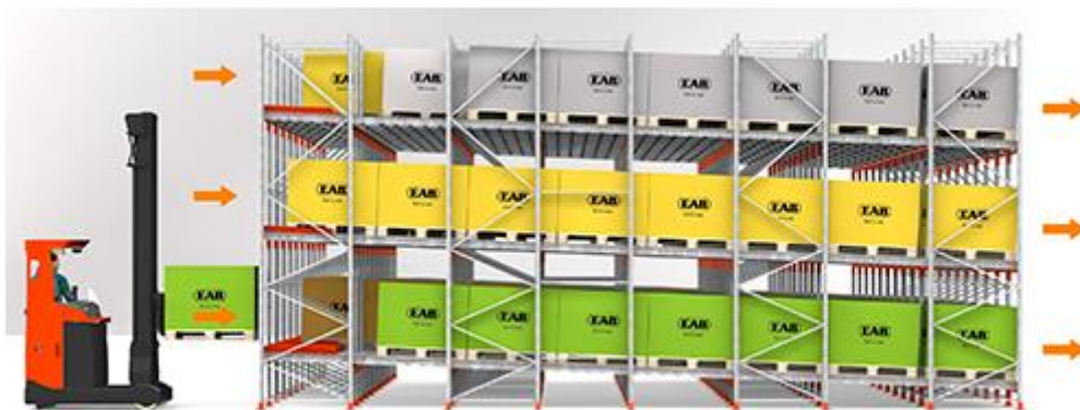
FIGURE 7. Operational principle of flow-through shelf (12)
