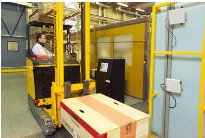
FIGURE 16. RFID system in inbound process in ABB (26)
