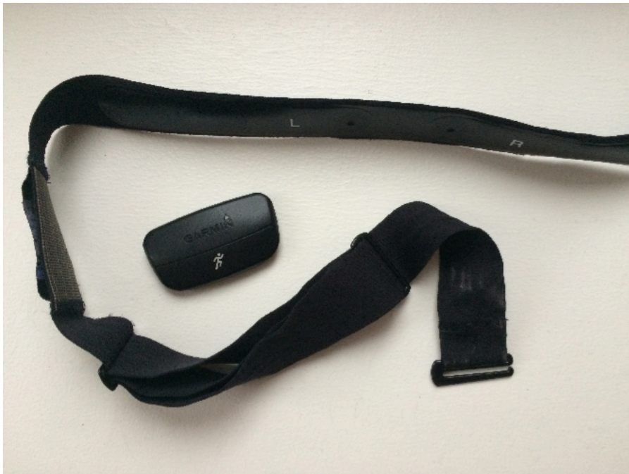
Figure 4. Electrode based HRM belt from Garmin.
