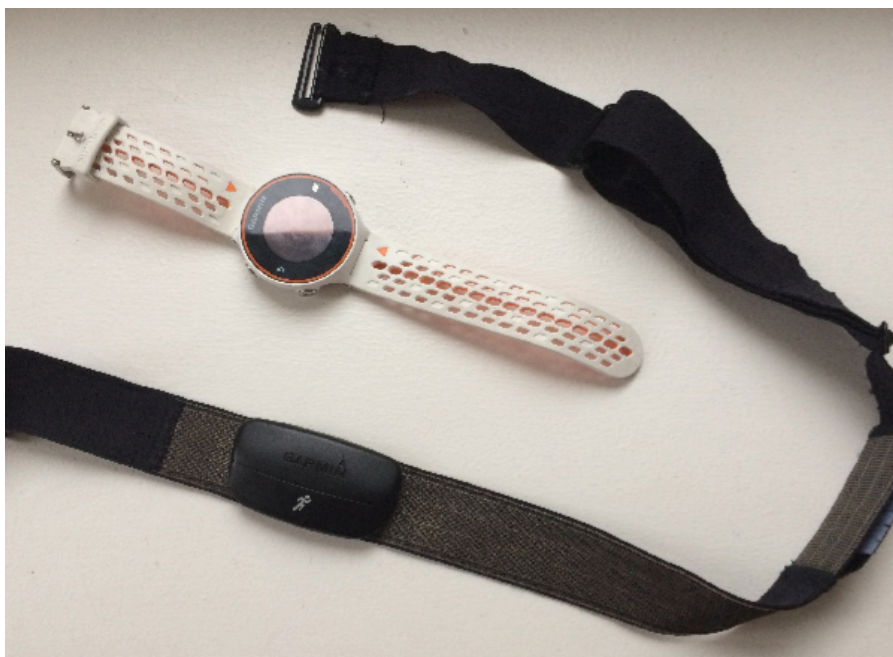
Figure 15. Garmin's Forerunner 620 wrist monitor and HRM-Run belt.
