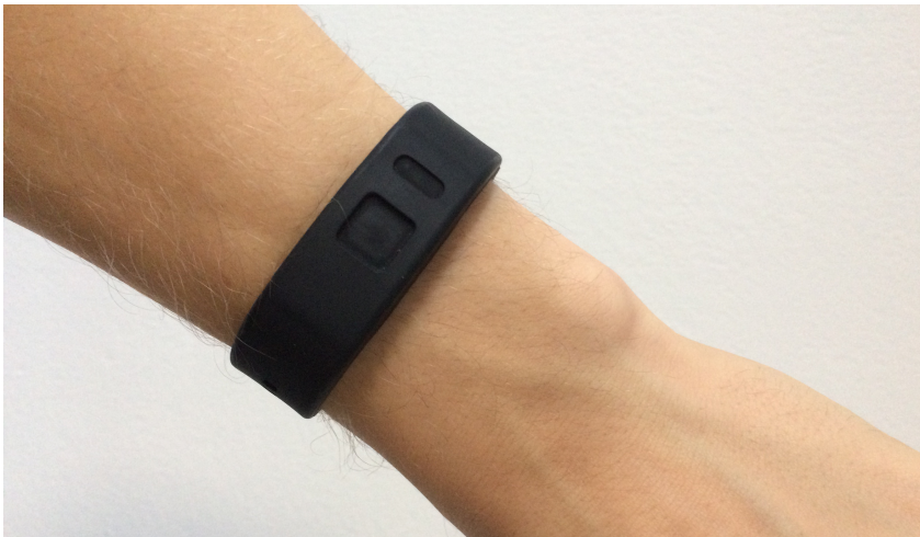
Figure 11. OHR Tracker is worn in the wrist, one finger's width from the wrist bone's peak.
