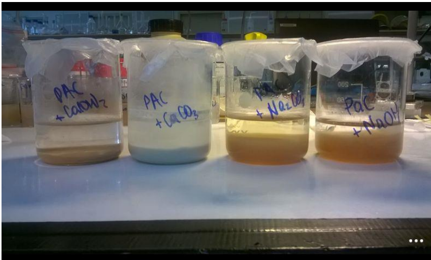
Figure 19. A comparison of different chemicals used for pH adjustment of the solution. From left to right – \text{Ca}(\text{OH})_2 , \text{CaCO}_3 , \text{Na}_2\text{CO}_3 , \text{NaOH} . The fourth sample (with \text{NaOH} as a neutralizer) was not settled completely when the picture was taken. The volume of sludge for this sample reduced twice after an hour of full settling time.
