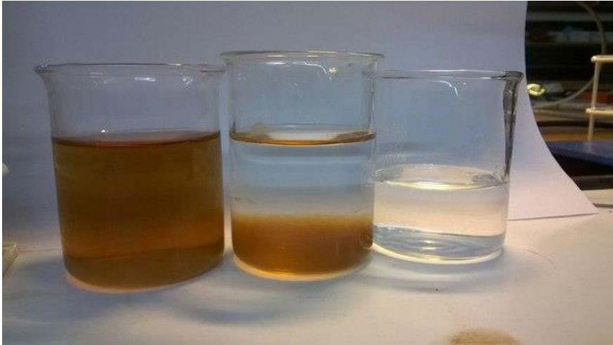
Figure 3. Chemical coagulation applied to HA synthetic water in this study. Left to right: a) 50 mg/L humic acid initial solution, b) after coagulation (PAC used as chemical coagulant) and flocculation, c) after floc removed by filtration.
