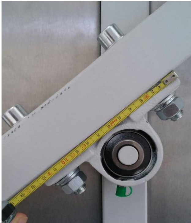
Figure 55 Rotating connection of door handle.
