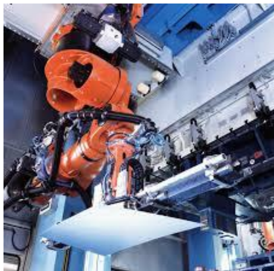
Figure 6 A crossbar robot holding sheet metal (Schuler n.d.).
