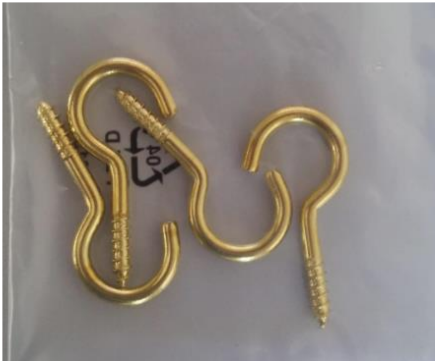
Figure 15 Commercial hooks used in manual transfer mechanism.
