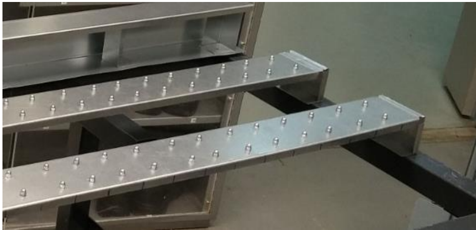
Figure 11 Dome shaped projections with nut as solution for cooling issue.
