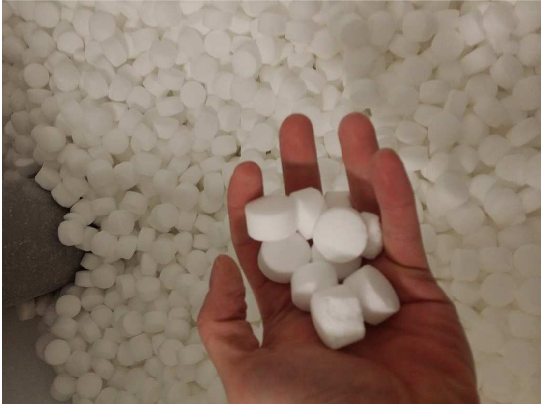
Figure 4 Large salt (NaCl) grains that are fed to the chlorine producer.
