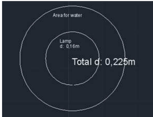
Figure 9 Visualization of UV-radiation chamber with tube and pipe dimensions.
