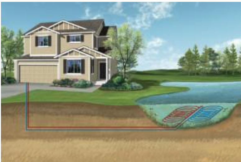
FIGURE 5. Lake closed loop system /5/
