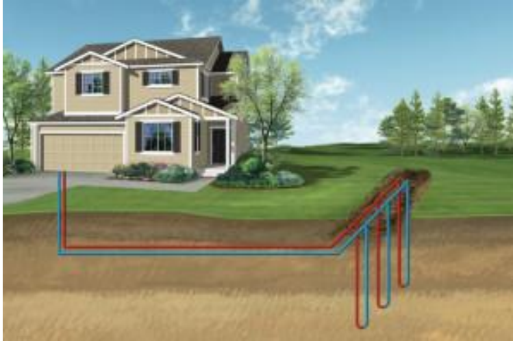
FIGURE 4. Vertical closed loop system /5/
