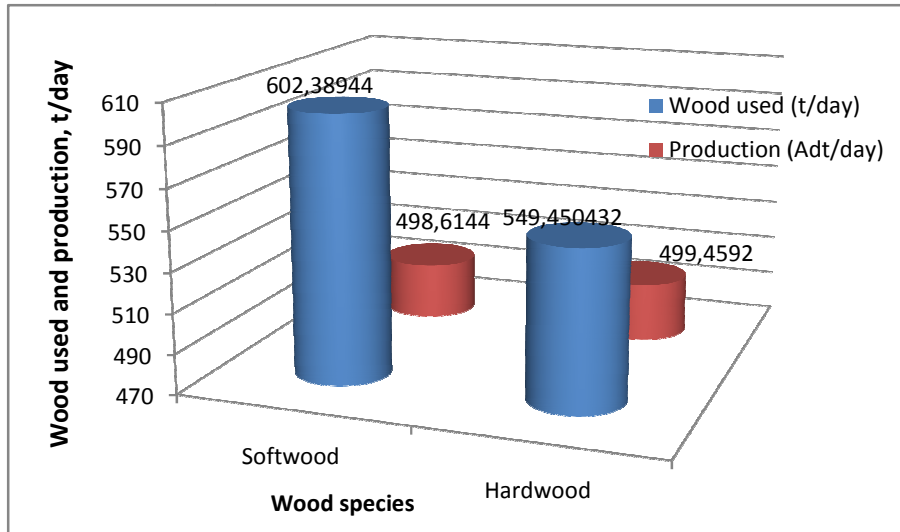
Chart 5.2 The consumption of amounts of wood used and pulp produced by CTMP process (Appendix 2)
