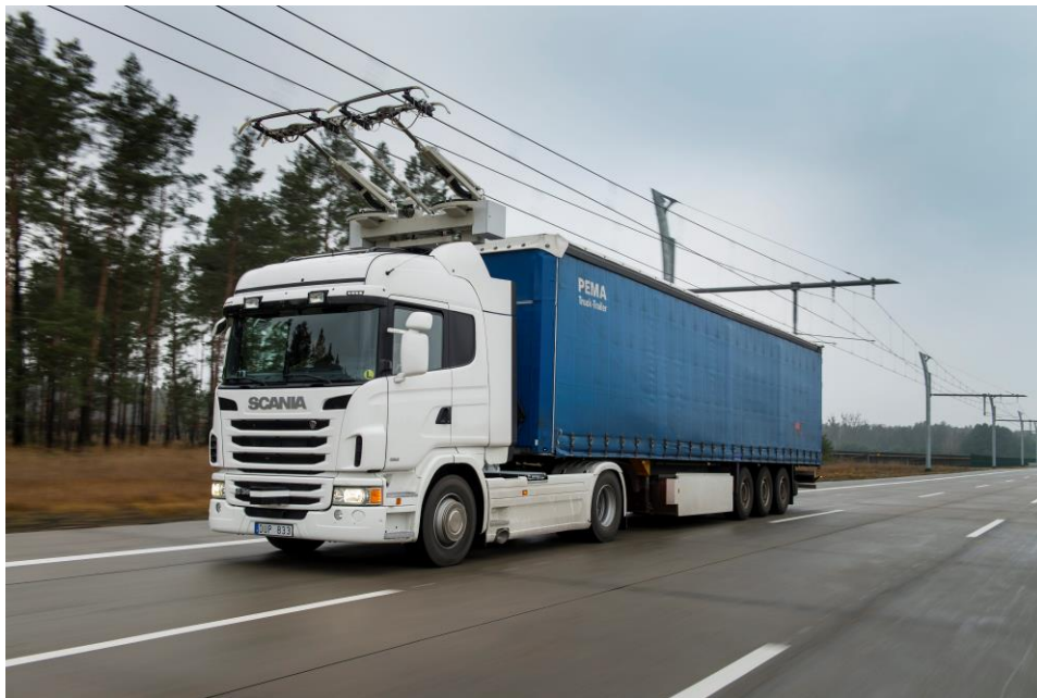
Figure 1. Scania lorry testing eHighway
